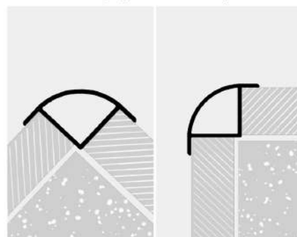
铺设方法示例Laying method example:
